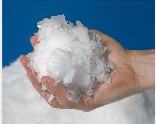
Use of Flaked Ice— for hot weather concreting (Fig. 03)
