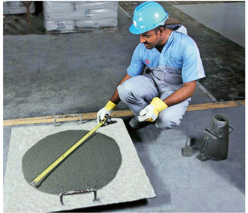
Flow test for self compacting concrete
